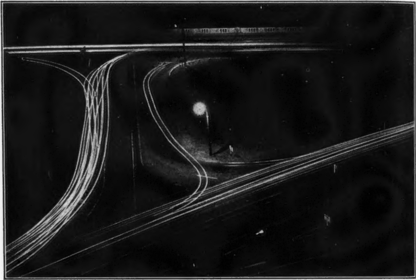
FIG. 3.—TRAFFIC MOVEMENTS TRACED BY PHOTOGRAPHING MOVING HEADLIGHTS. NOTE ONE WRONG ROUTE NEAR CENTRAL LIGHT
